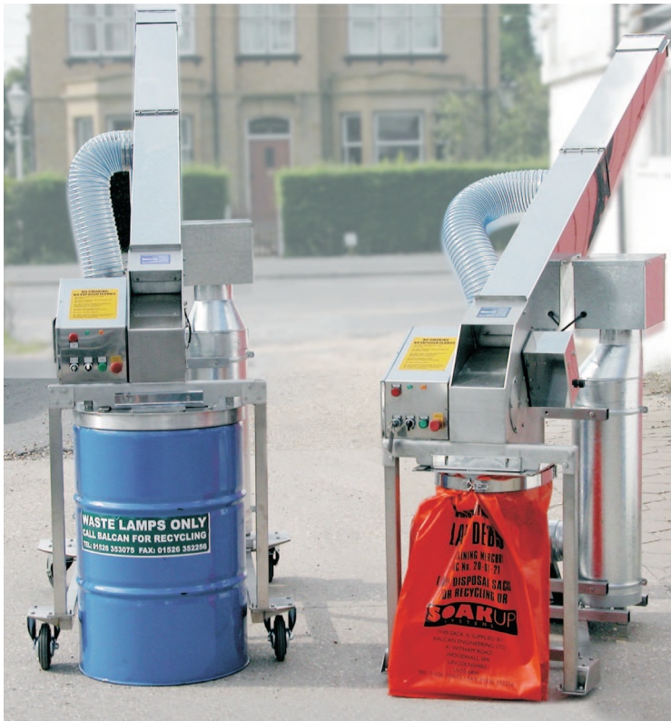
Balcan Electric Lamp Crushers available with Sack System or Drum Adaption.
