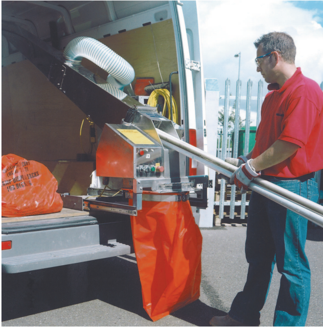
The Balcan Low Loaded Lamp Crusher in use whilst supported on it's sliding rails.
