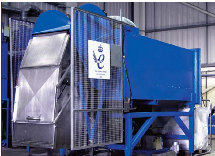
Loading of the Recycler is by means of the hydraulically operated stainless steel loader mounted on the front which accepts either 210 litre drums or loose debris. This photograph was taken whilst in actual use within Balcan
