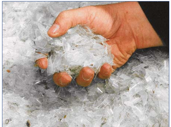
After going through the Balcan Recycler MPC4000 the clean glass cullet is not so sharp so can be handled with care.
