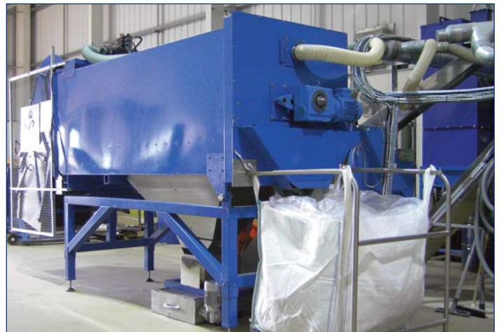
This shows the other end of one of the two Separators from where the metal and plastic components are discharged and collected. Two of these are used in parallel.
