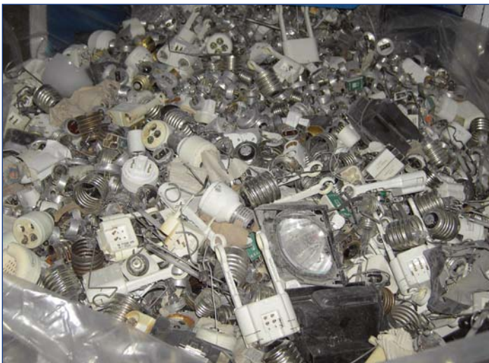
Examples of the type and condition of the metal and plastic debris separated from the glass of the waste lamps.
